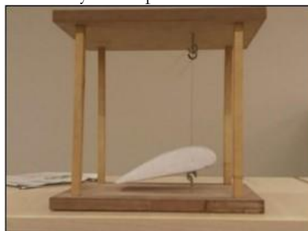
Figure 7 - Device with aerodynamic profile GÖ387 for vertical displacement.
