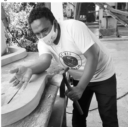
Figure 3 – Master Otávio building a cave with the adze
